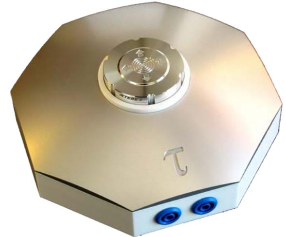
The instrument is powered by a **CR1612 lithium battery** that has to be precautiously exchanged every two years to keep the device in perfect efficiency.
